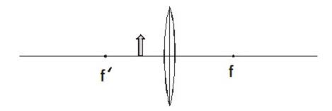
**10.** Construct the image formed by the object as shown below. If the focal length of the lens is 15.5 cm and the 3.20 cm (in height) object is placed 22.0 cm from the lens, find (a) the image distance, (b) the magnification, (c) the image height.
